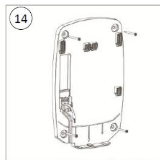
Screw the Plug-in base to the wall(x4)
