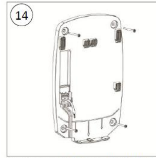
Screw the Plug-in base to the wall(x4)
