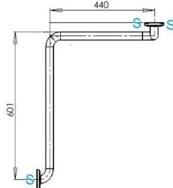
It is recommended to set up the horizontal part of the bar between 700 and 750 mm height, with respect to the ground.
