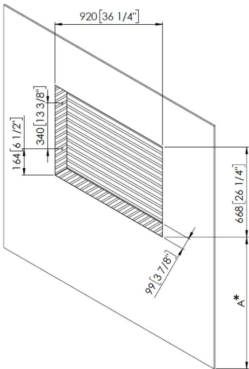
Make required the wall cut according to the drawing
